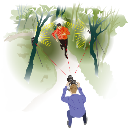
With the WR-R10 attached to the D7500 as a commander, three SB-5000 Speedlights are triggered wirelessly via radio.
